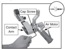
Figure 3. Installing the contact arm.
